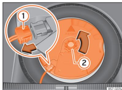
**Fig. 242** Na bagageira: desmontar o subwoofer.
