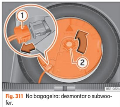
**Fig. 311** Na bagageira: desmontar o subwoofer.
