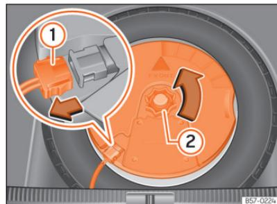
**Fig. 222** Na bagageira: desmontar o subwoofer.
