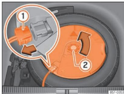
**Fig. 239** Na bagageira: desmontar o subwoofer.
