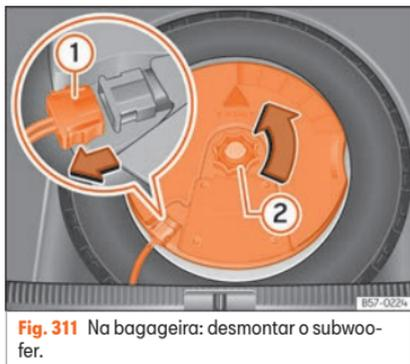
**Fig. 311** Na bagageira: desmontar o subwoofer.
