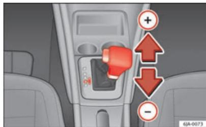
Fig. 106 Alavanca selector: Tiptronic
