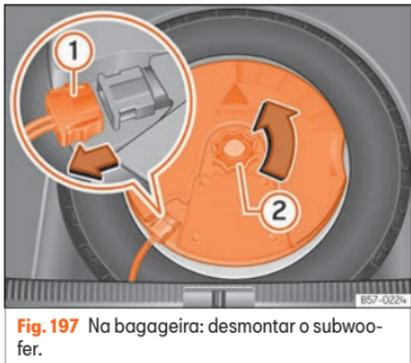
**Fig. 197** Na bagageira: desmontar o subwoofer.
