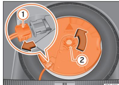
**Fig. 218** Na bagageira: desmontar o subwoofer.
