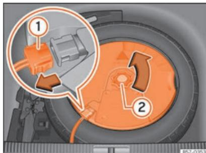
**Fig. 232** Na bagageira: desmontar o subwoofer.
