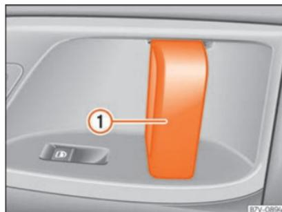
Fig. 98 Na porta de correr.: manípulo da porta
