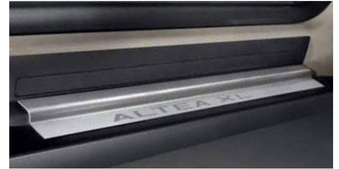
Juego de estriberas logo ALTEA XL en acero inoxidable, protegen el paso de puerta de golpes y arañazos. Set of footrests, with ALTEA XL logo, in stainless steel to protect the vehicle from bumps and scratches when getting in and out of the car. Jogo de forras de embaladeira logo ALTEA XL em aço inoxidável, protegem a embaladeira de impactos e riscos. 5P8071500
